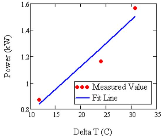
Figure 8: Comparison between the recovered power from the heat exchanger and the difference between the temperature of the hot waste shower water and the cold faucet temperature for the cold, warm, and hot shower tests. A best fit line is also plotted.
