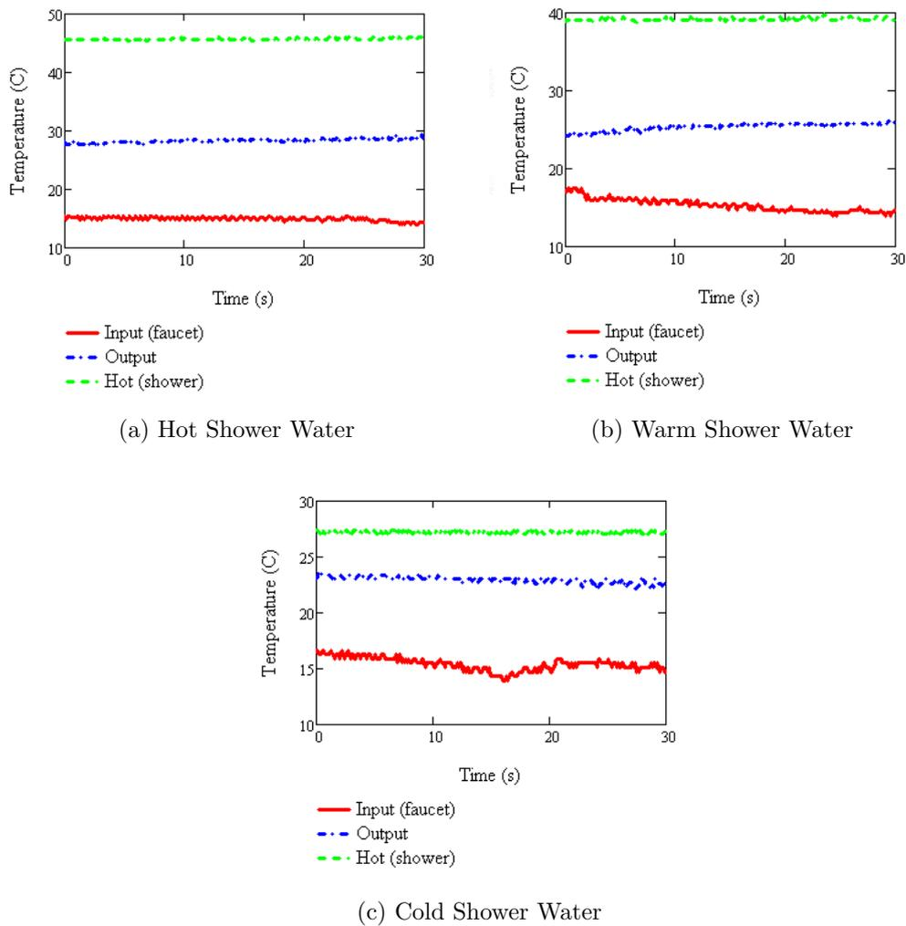
Figure 7: Thermocouple readings with three different temperatures of waste shower water.
