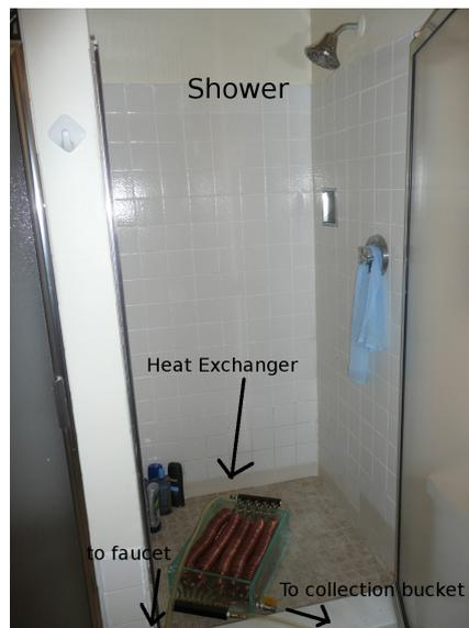
Figure 6: Experimental setup. Heat exchanger has clear tube connected to faucet (not pictured) which splits into ten parallel, coiled copper tubes. Shower water was sprayed on the copper tubes which then recombine. The cold faucet water travels through the copper tubes and is heated up by the shower water. The heated cold faucet water is collected in a bucket.
