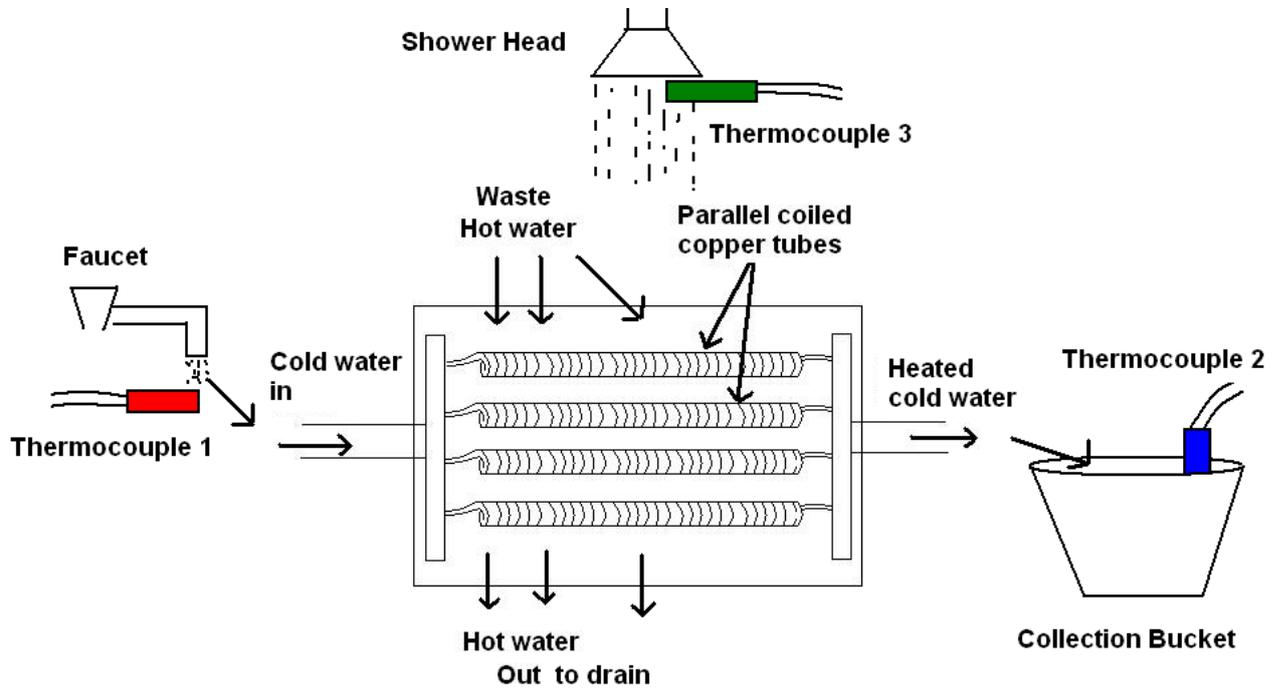
Figure 4: A schematic of the experimental setup used in this experiment. The input tube is connected to a faucet which provides cold water. The cold water is pumped through the coiled copper tubes of the heat exchanger. Hot waste shower water is sprayed over the copper tubes. The heated cold water then is collected in a bucket.
