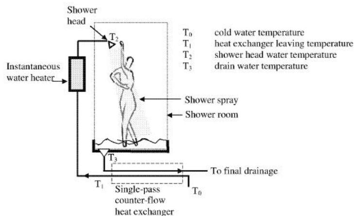
Figure 9: A possible installation for a counter-flow heat exchanger tested by Wong, etc. The hot drain water is used to heat the input water, which is then further heated by the instantaneous water heater. This provides significant energy savings.<sup>5</sup>
