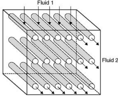
Figure 3: Cross flow heat exchanger. This is a simplified version of the actual heat exchanger used in the experiment, with the difference being that the tubes that fluid 2 flows through are actually spiralled, which gives a larger surface area in contact with fluid 1 and therefore a better heat exchange.<sup>1</sup>
