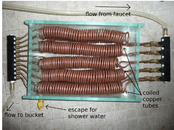
Figure 5: Close up of heat exchanger. The copper tubes are stacked five wide and two deep. The valve pictured bottom left is for the drainage of the hot shower water. It was kept open during the experiment so hot shower water flowed over the copper tubes and out the valve to the drain.
