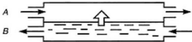
Figure 1: Simple design of a recuperator. Fluid B is at a higher temperature than fluid A, and heat is transferred across the boundary.<sup>1</sup>
