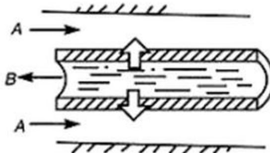
Figure 2: Transmural heat transfer. The heat from fluid B first passes through the walls of the pipe before being transferred to fluid A.<sup>1</sup>
